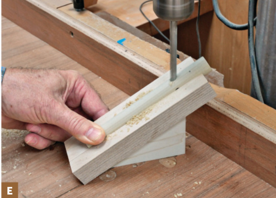
E Position a trunk in the jig and drill holes where you want them for the branches. Brad-point bits prevent wandering as you start the holes.
