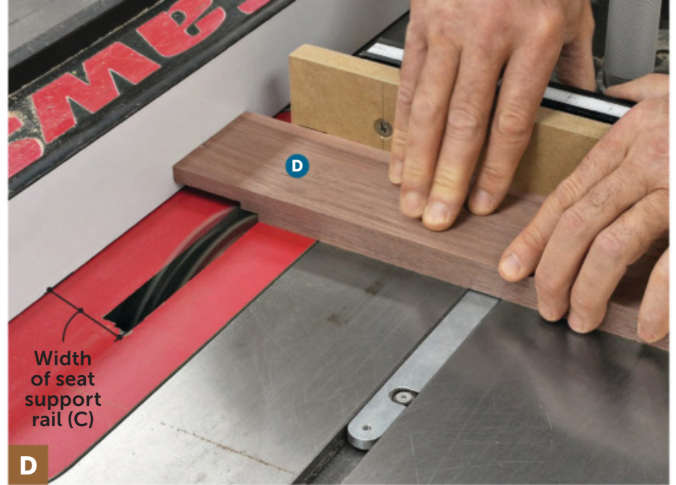
D Attach an auxiliary fence to your miter gauge to back up the cut. Make several passes over the dado blade until the end of the seat support stretcher (D) touches the rip fence.
