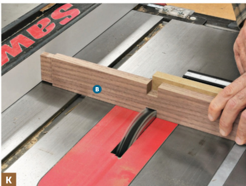
K Use the rip fence as a stop to position the leg rail (B). When cutting the second notch, butt the same end of the rail against the fence to ensure the notches align perfectly.
