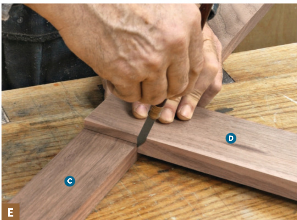
E Place a seat support rail (C) on your bench with the rabbets up. Center the rabbet of a seat support stretcher (D) on the length of the rail. Mark along the edges of the stretcher with a marking knife.
