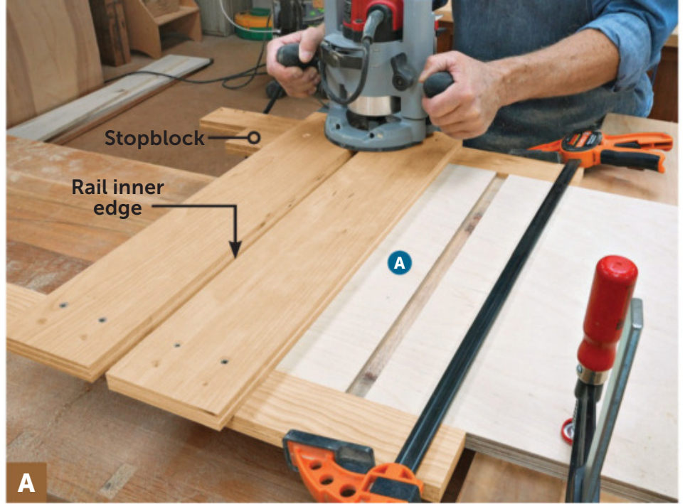
Screw a stopblock to the underside of the jig with one end flush to the inside edge of a rail. Position the jig with the stopblock touching the end of the side (A), clamp it in place, and rout the rabbet.
